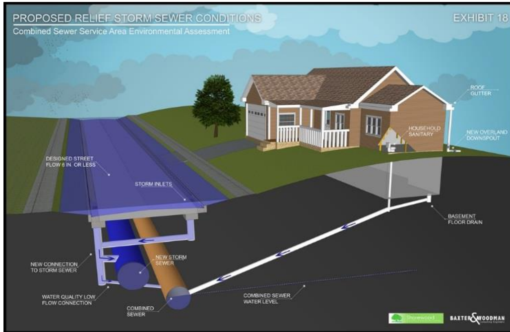
Figure 4: Proposed Conditions Portrayal of a Virtually Separated Combined and Storm Sewer System. The flow into the combined sewer is restricted, keeping water levels low inside the sewer, and the overflow is re-routed to the storm sewer.
