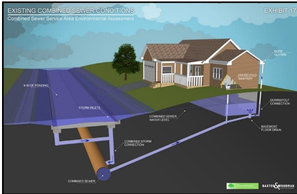
Figure 3: Existing Conditions Portrayal of a Surcharged Combined Sewer System. Basement backups occur when the water level in the combined sewer is higher than the sanitary sewer service and basement.
