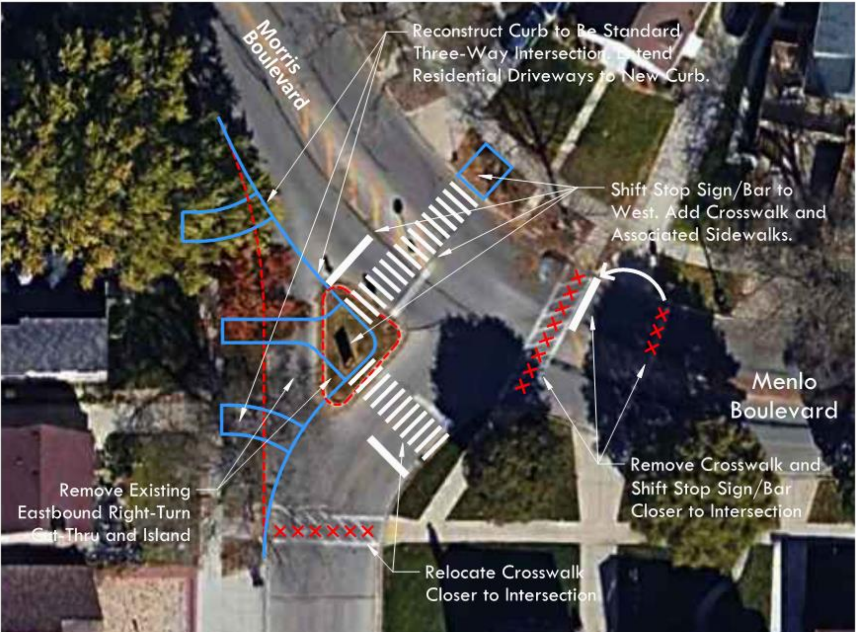
Exhibit 20: Morris and Hubbard Intersection Recommended Improvements
